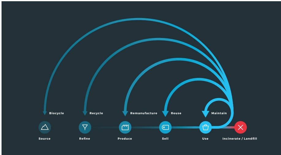
Figure 12.1: Circular ‘cascading’ activities (i.e. maintain, reuse, refurbish, recycle) can be used to slow, close and narrow the loop.
